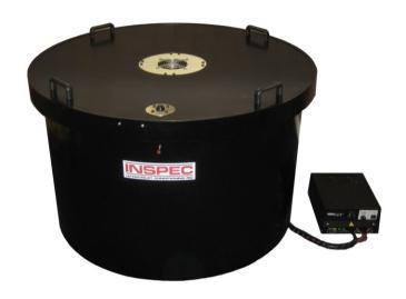
Specimens are held in "finger" clamps (which are supported on a number of concentric hoops positioned at various heights), so that the specimens are facing inwards towards the radiation.
