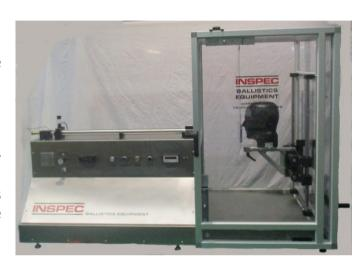
The rig is capable of a projecting a 6mm diameter steel ball at a range of velocities from 12 - 200 m/s.
